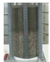
No.1(Bor-3,4) 判定B 浸透層厚12mm
